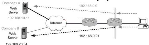
Refer to the exhibit above. The Certkiller administrator wants a user on the inside network to access two sites on the Internet and present two different source IP addresses. When the user is accessing Company A's web servers, the source IP address is translated to 192.168.0.9. When the user is accessing Company B's web servers, the source address is translated to 192.168.0.21.
