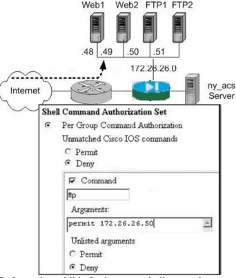
Refer to the exhibit. In the network diagram there are four servers on the DMZ; two web servers and two FTP servers. According to the group configuration in the ny\_acs server, when a remote user accesses the security appliance and is authenticated, the user is authorized to perform which two actions? (Choose two)
