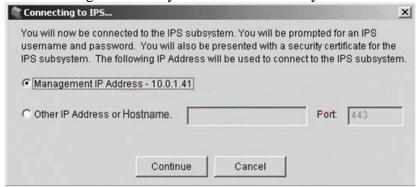
Refer to the exhibit shown above. When accessing the IPS icon in ASDM, the administrator is presented with a "Connecting to IPS" popup window. In the window, the management IP address A.B.C.D is displayed where A.B.C.D is an actual IP address.
