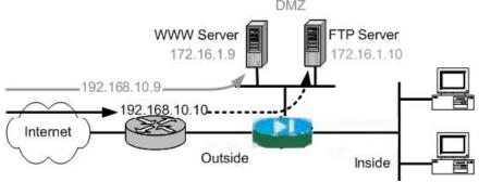
Refer to the exhibit shown above. The Certkiller administrator wants to permanently map host addresses on the DMZ subnet to the same host addresses, but using a different subnet on the outside interface. Which command (or set of commands) should the administrator use to accomplish this?
