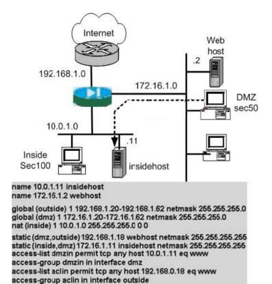
Refer to the exhibit above. Users on the DMZ are complaining that they cannot gain access to the inside host via HTTP. What did the network administrator determine after reviewing the network diagram and partial configuration?
